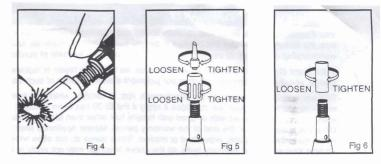
Remove brass burner assembly and squirt 2 shots of butane into orifice to clear any debris
